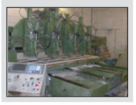
ProCut bring out the Shoda 4 head router for those job's that can't be stacked and with 4 piggy backed drilling heads makes short work of any
